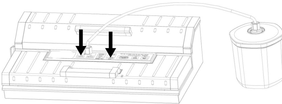
Insert one end of the hose into the air intake and another end of the hose into the center hole of the canister cover.
