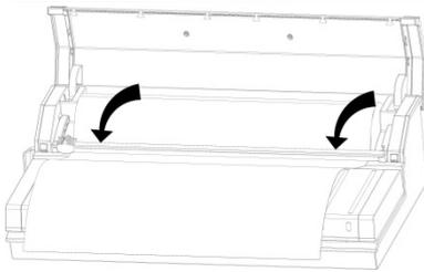
Put down the cutter rack and make sure it is on the right place of the bags, then slide the cutter from one end to the other end to cut the bag.
