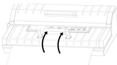
Press the “**Vakuum & Schweißen**” Button. The Vacuum Indicator Light, then the Sealing Indicator Light with light as the bag is automatically vacuumed and sealed. Once it is finished, both lights will turn off.
