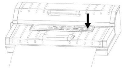
Press “Schweißen” (seal) button to start sealing the bags.
