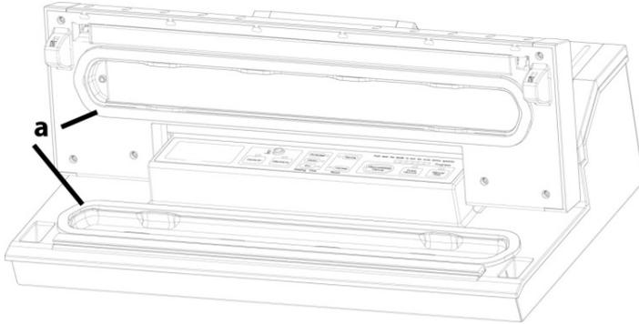
Turn off the device using the main switch. Let the device cool down completely. Open lid of the device. Take the upper/lower gasket out of the trough in the cover of device/from the trough around vacuum chamber.
