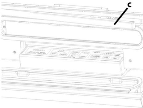
Take a new sealing bar and press the sealing bar into the trough again and check the position. Replace the clips on left and right side.
